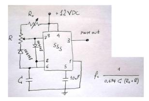
Values for R, R0 and C are given in a moment. The diodes are 1N4148. An explanation of the circuit will be given also below. Anyway, the idea is that by turning the potentiometer R, one can change the duty cycle, but the overall frequency does not change. This is because what is gained by the ON time is lost by the OFF time, and the total period of the signal is constant. The resistor R0 is used to tune the frequency (components have a certain deviation from the ideal values).
